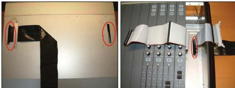
Fig 2-13 : Mixer Bus Cable Slots.
