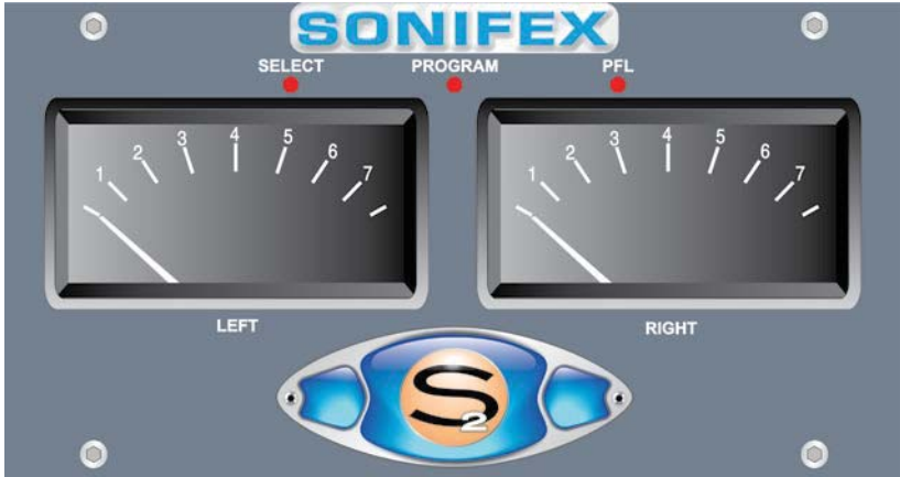
Fig 20-4: PPM & True PPM Meter Panel.
